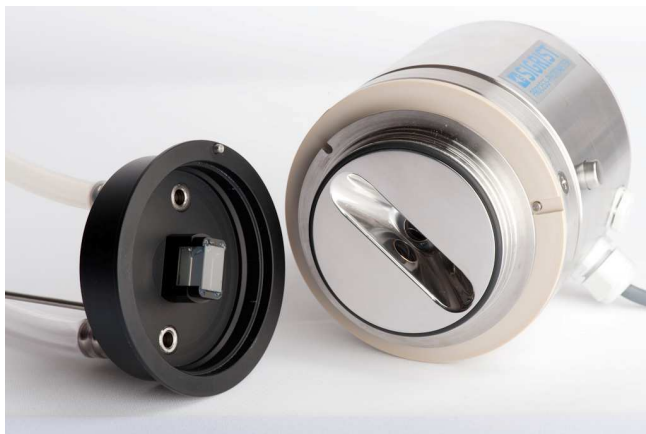
Checking unit with secondary standard Example TurBiScat
