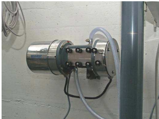
Measurement using a photometer “ColorPlus” from Sigrist-Photometer
