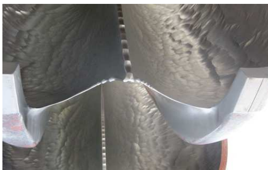
Fig. 2: Pelton turbine runner affected by abrasive erosion
