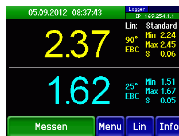
Picture 3: Measurement display with minimum/maximum values as well as standard deviations
