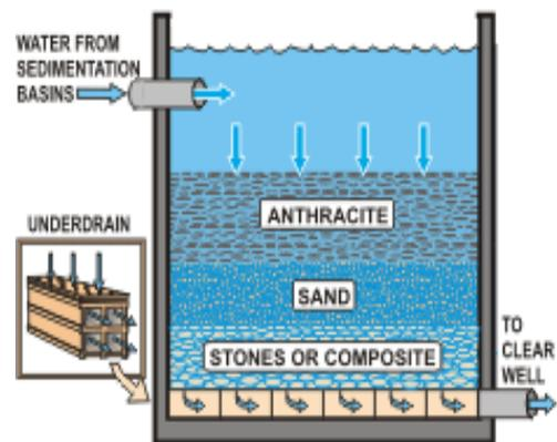
Example of a multilayer sand filter
