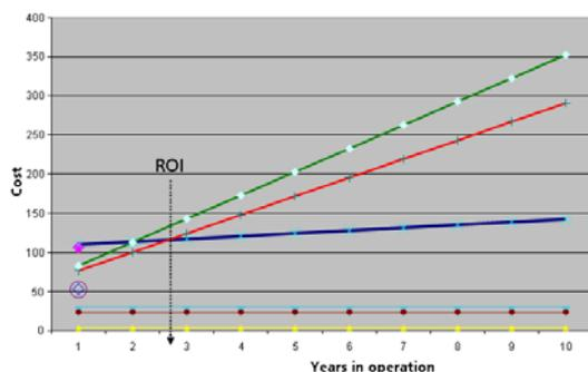
This example was calculated by a customer from England. The diagram shows at the bottom the annual operating costs of the AquaScat (yellow) and two evaluated comparative instruments (brown and light blue).
