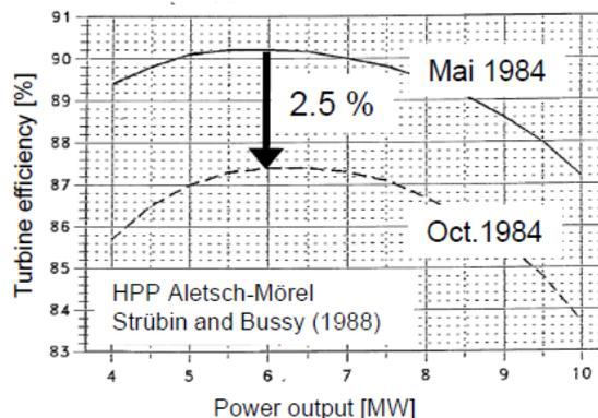
Fig. 3: Turbine efficiency reduction caused by abrasive erosion
