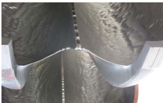
Fig. 2: Pelton turbine runner affected by abrasive erosion
