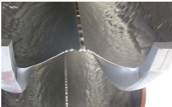
Fig. 2: Pelton turbine runner affected by abrasive erosion
