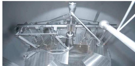
Picture 2: Lauter tun with raking device
