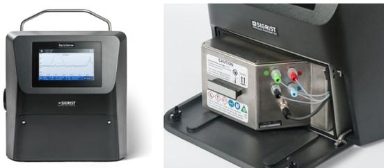
**Figure 4:** BactoSense with cartridge
